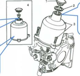
Fill the dashpot up to about 15 mms from the top of the cover. If you put in too much it will overflow when you replace the Dashpot assembly.
